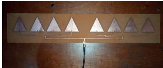
Gambar 12. Fabrikasi antena Arary 8x1
