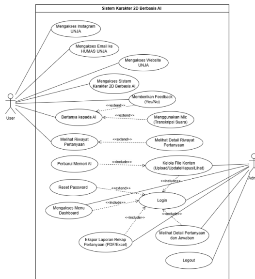
Figure 3. Use Case Diagram Sistem
