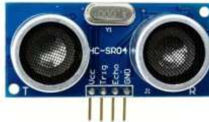
Gambar 4. Sensor Ultrasonic HC-SR04.
