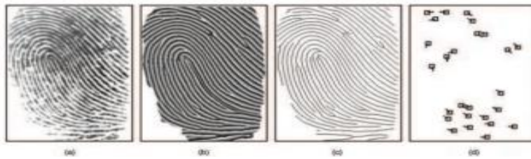
Gambar 1. Skema representasi sidik jari. (a) Grayscale image (FVC2002 DB1, 19_1), (b) phase image, (c) skeleton image dan (d) minutiae (Feng & Jain, 2011)
